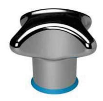
DH 302 Stainless Steel Four lobe knobs are intended for use in hygiene areas. The sealed mounting surface enables fastening without dead spaces. The high quality finish as well as the large corner radius and closed surfaces prevent adherence of dirt and facilitate cleaning.
