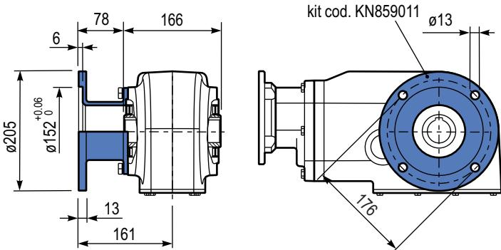
**PX73NBR..** Reaction Arm
