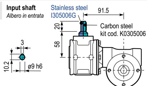
P3D3 SMA... Single output shaft
