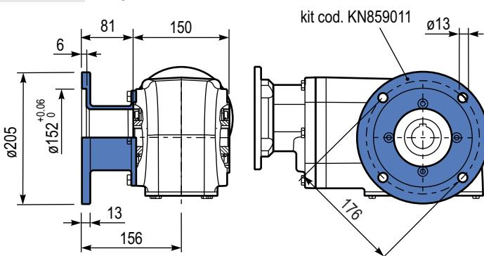
**PX62NBR..** Reaction Arm
