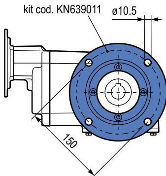
**PX43NBR..** Reaction Arm
