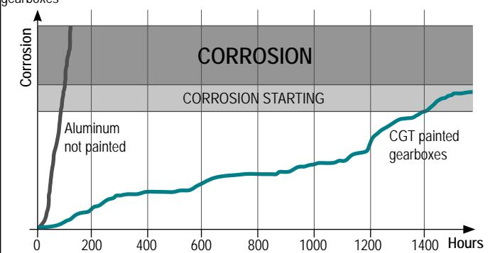
This graph is an indication, since some chemical components may be more aggressive than the salt spray test. Tests are suggested on special cases (in case use type "N series", full stainless steel gearboxes).
