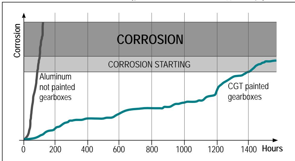
This graph is an indication, since some chemical components may be more aggressive than the salt spray test. Tests are suggested on special cases (in case use type "N series", full stainless steel gearboxes).
