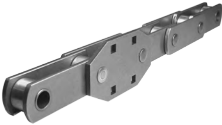
152.4mm pitch bucket elevator chain w/ G4 attachment with square holes for captive bolts
